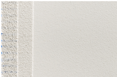
BASWA Cool Classic Top Base coat Base / Base Cool 0,7 mm Finish coat Top 0,3 mm
